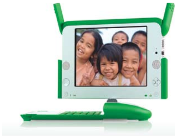
OLPC computer designed by Fuseproject. This laptop has a swivel top so that the computer screen can lie flat or be tilted. In a Nigerian village, a girl carries her laptop .
